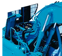
Service bonnet has gas damper cylinder for easy opening.
