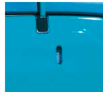
Hydraulic oil gauge shown against white background for easier reading.
